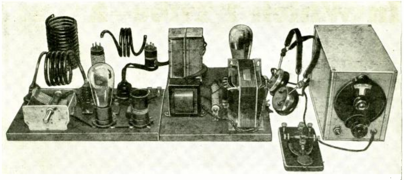
Front view of the C.W. (code) amateur transmitter, which is here described in detail by Mr. Victor, together with its power supply unit.
