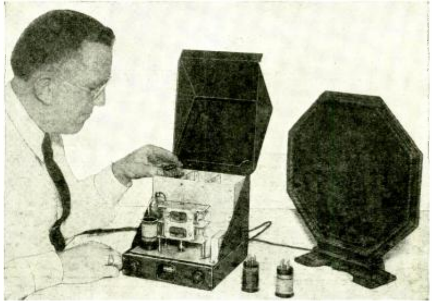
It's "dead easy" to change the plug-in coils in the Leotone receiver, thanks to the diagonally opening metal cabinet. This 4-tube, 2-volt receiver operates a loud speaker nicely.
