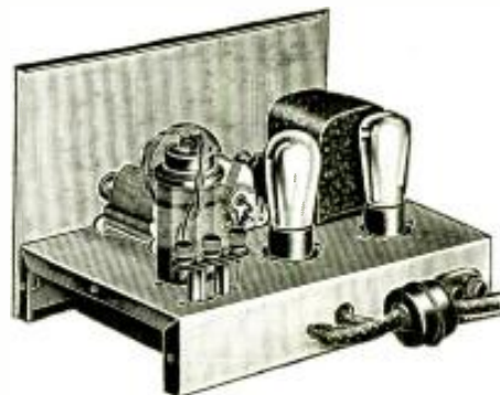
Rear view of the receiver, showing the new type tuning coil.
